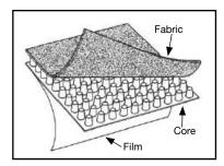
The Drain Max 520 Series is designed for use with the Drain Max water-proofing systems in vertical installations requiring high compressive strength and flow capacity. Use is suitable in selected horizontal applications.
